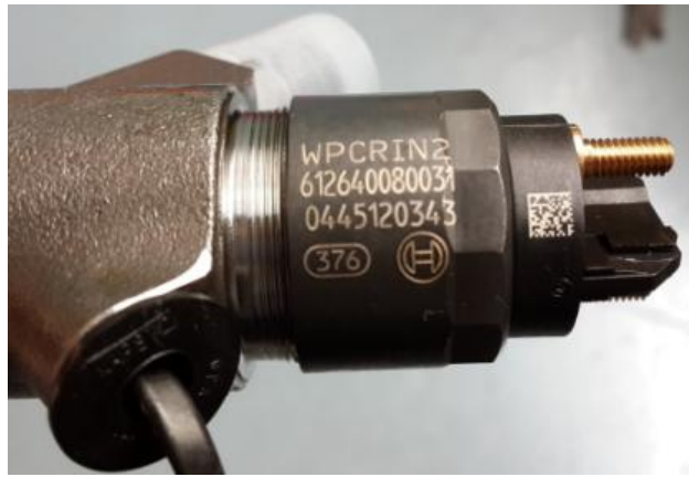
Figure 4-55 Fuel injector marking specification
